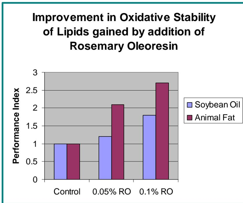
Stability is determined by an OSI Instrument at 110° (The OSI induction time of the fortified sample divided by the OSI induction time of the Control).
